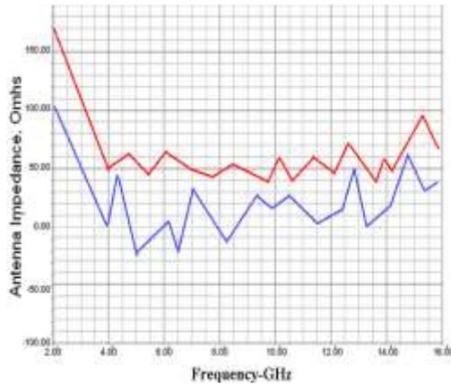
Fig. 1(c) : Antenna impedance versus frequency (real part → red color and imaginary part → blue color) of circular Planar UWB monopole Antenna.
